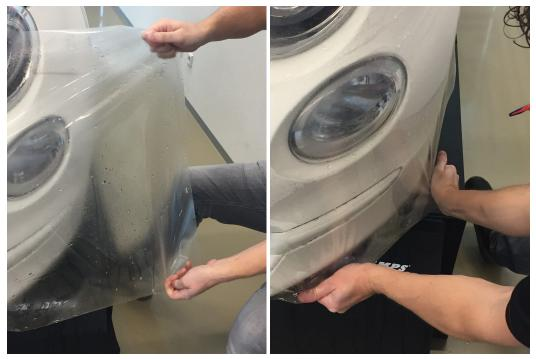
Conventional convex and compound shapes on car fronts are mostly suitable to be covered with Avery Dennison SPF-XI Paint Protection Films, but in some deeper corrugated shapes it may be necessary to make an incision in order to avoid any form of air/water entrapment in the deep recesses. This incision does not jeopardize the functionality or durability of the product.
